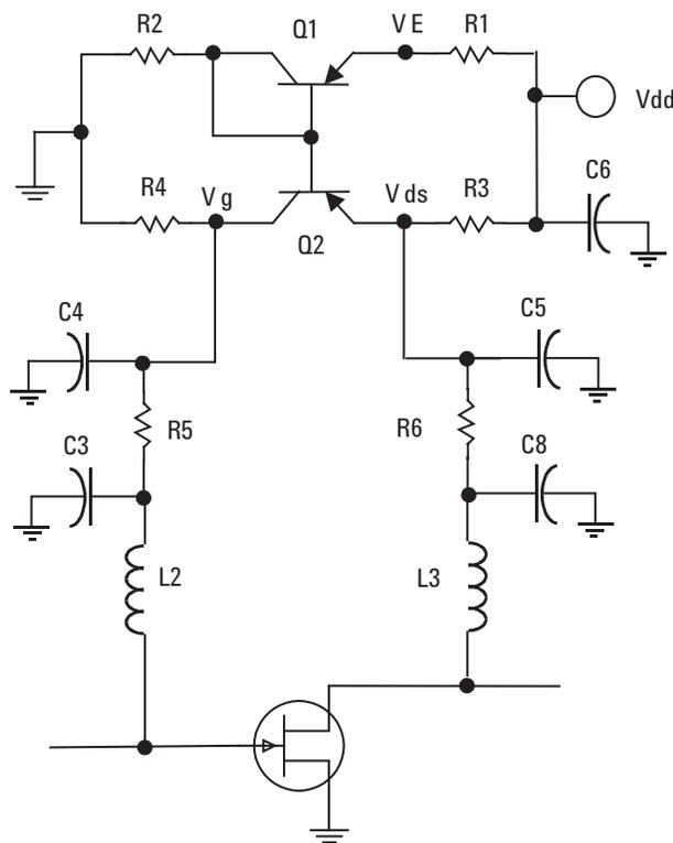
**Figure 17. Typical active bias applied to a FET transistor**
