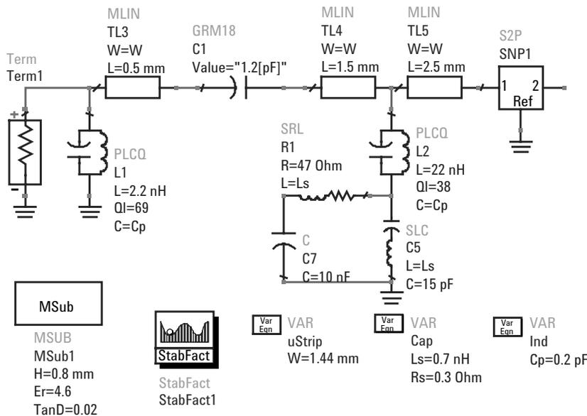
Figure 5. Input matching & biasing networks
