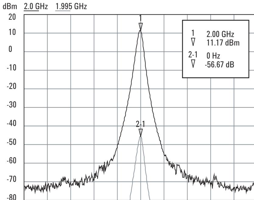
Figure 14. Fundamental tone and lower intermodulation product overlaid over the same freq. axis
