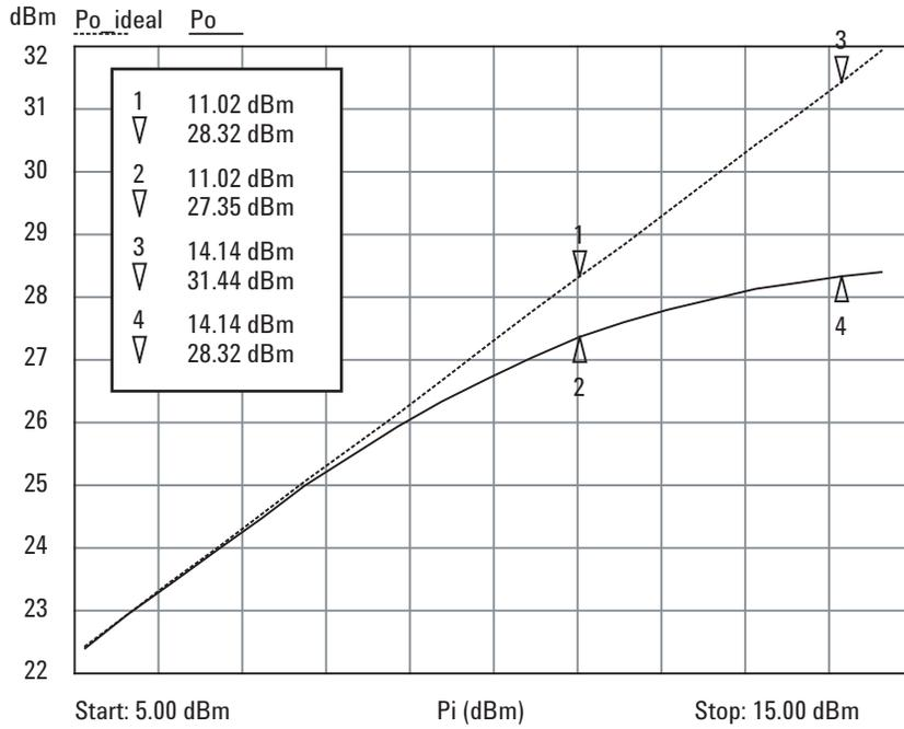
Figure 12. Theoretical & Measured Output Power Vs. Input Power
