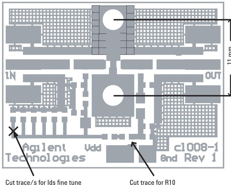
Figure 4. Positions of PCB trace cuts and distance between heatsink screws
