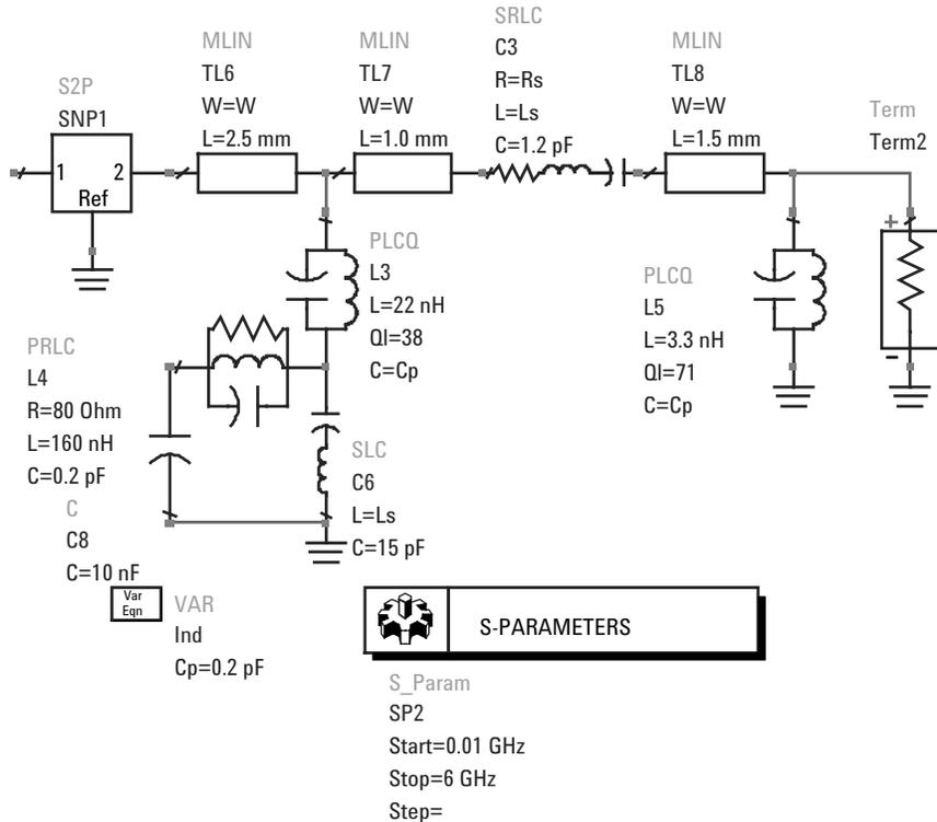
Figure 7. Output biasing and matching circuit
