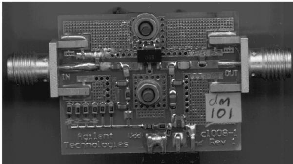
Figure 2. Fully assembled demoboard with PCB-edge mounted SMA connectors
