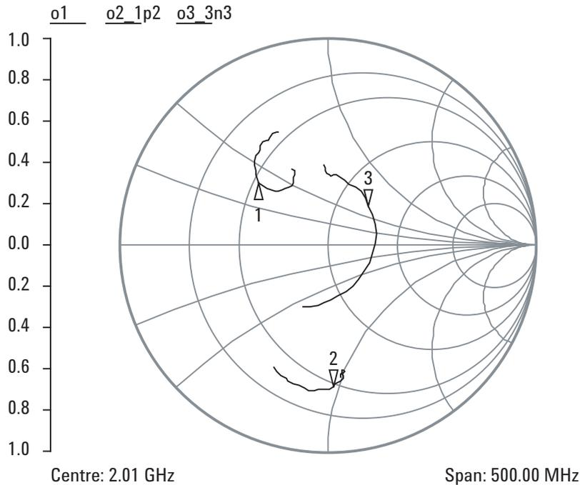
Figure 8. Measured trajectories of output impedance during the various phases of matching
