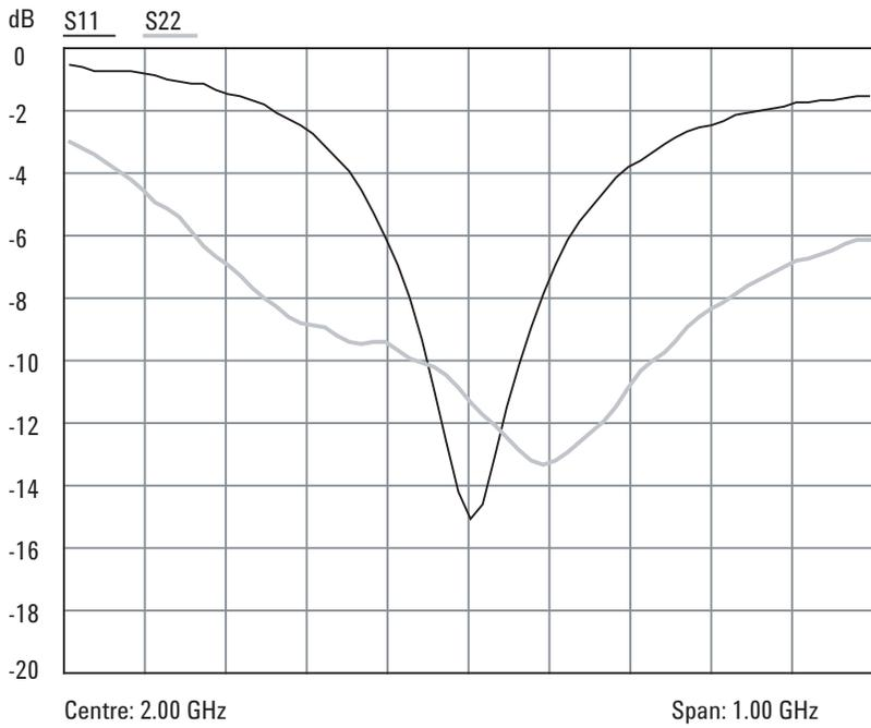
Figure 10. Measured input and output return loss
