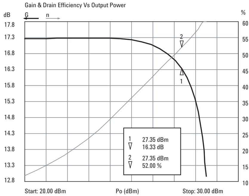
Figure 13. Measured gain vs. output power
