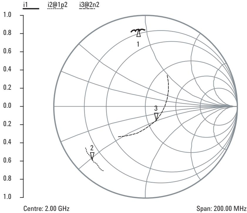
Figure 6. Measured trajectories of input impedance during the various phases of matching
