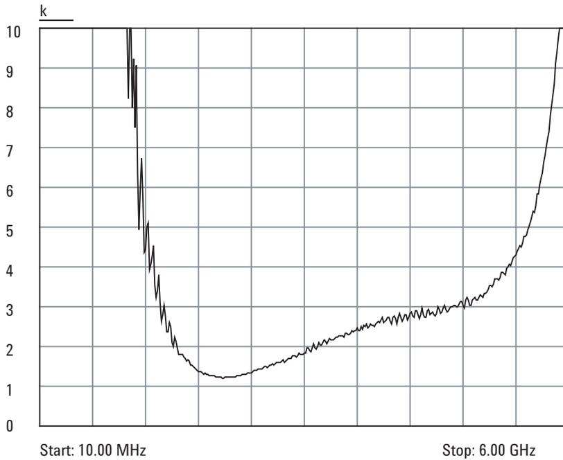
**Figure 15. Stability (k) calculated from measured s-parameters**
