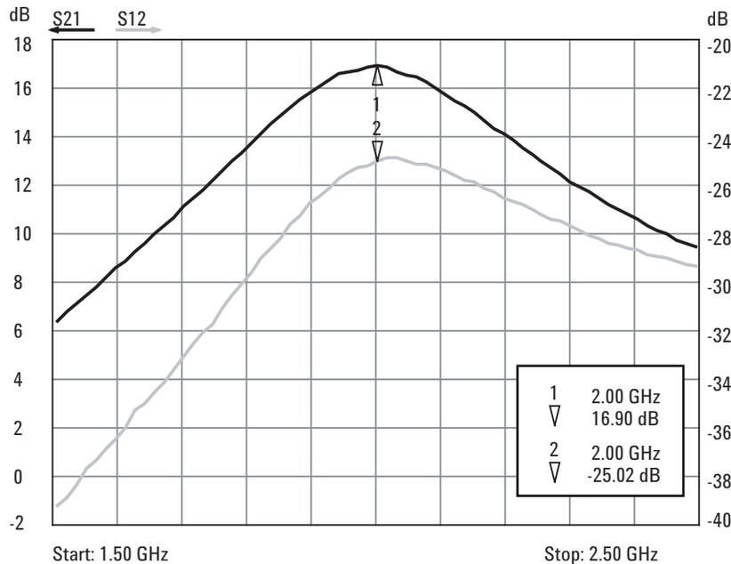
Figure 11. Measured forward gain and reverse isolation
