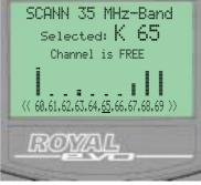
Display for selecting the transmitter channel
